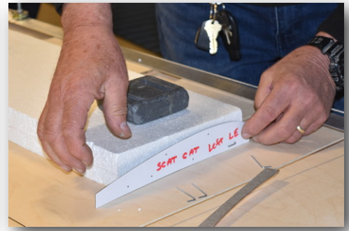
Setting up to cut top of airfoil.
