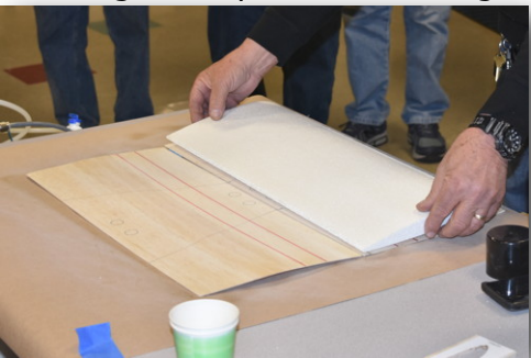
Attaching sheeting to core.
