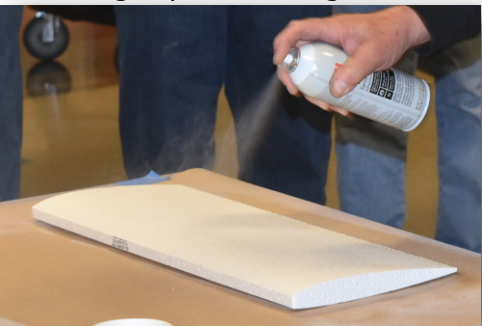
Applying adhesive to foam core.
