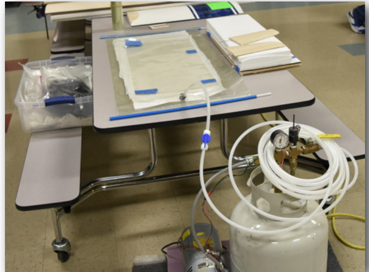
Craig's vacuum bagging equipment.
