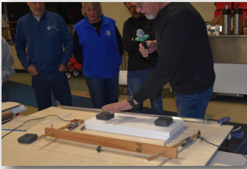
Bottom of airfoil cut half way there.
