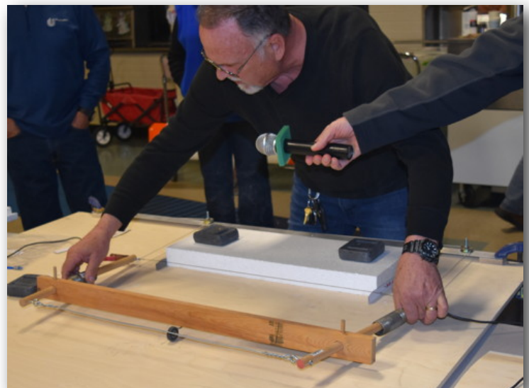
Craig starts the cut with the bottom of the airfoil.
