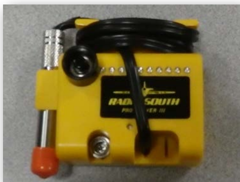
Hank's glow plug driver / tester
