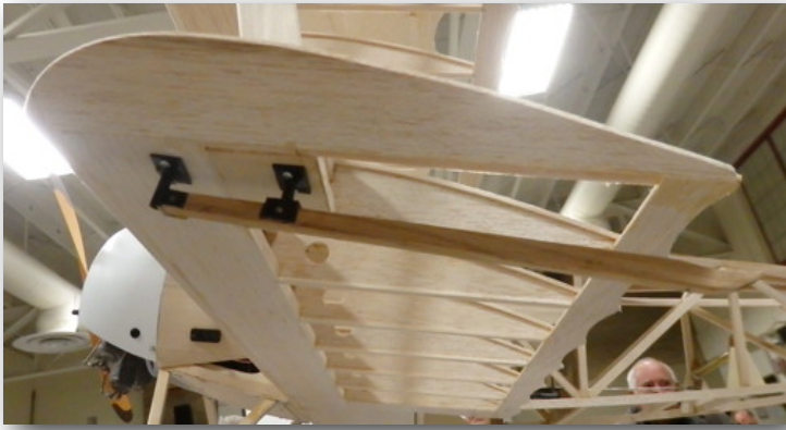
Bruce's wing skid detail. These planes were prone to tipping with their narrow landing gear spacing.
