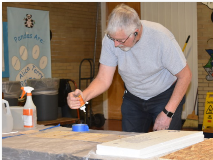
Paul applies a sparing amount of Gorilla Glue to bind the sheeting to the foam core.
